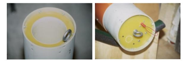
This is the forward end of the fin can showing the G10 coupler and centering ring. Note the 12 bolts holding the fore and aft retaining rings, which provide a sturdy attachment for the centering ring.
