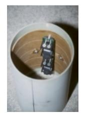
The main electronic control for recovery is a Black Sky Research AltAcc, which uses an accelerometer for determining drogue deployment, and a pressure transducer to determine the proper altitude for main parachute deployment. Backup electronic control is via second AltAcc or a BSR timer. The timer will be programmed with deployment times determined by computer simulation, and will control it's own separate ejection charges.
